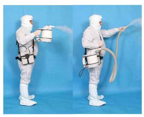
The convenient shoulder and hip harness allows the technician to carry the Portable Fogger and conduct fog tests without a trailing power cord, switching between a **TRIGGER MODE** or **CONTINUOUS MODE** can providing an "On Demand" fog or continuous fog. The airflow can be switched from low to high, just as easily as the mode of operation. The Portable FogGun is conveniently attached to the shoulder harness/battery pack frame for hands-free testing.
